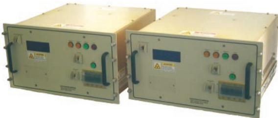
The front panel had the same operating points, however, a vacuum fluorescent display was added to improve operation and diagnostic processes. ETM is now in production of hundreds of these power supplies to support the program.
